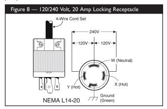
This receptacle powers 120/240 Volt AC, 60 Hz, single phase loads requiring up to 2,400 watts of power at 20 Amps for 120 Volts OR 4,200 watts of power (4.2 kW) at 17.5 Amps for 240 Volts. The outlet is protected by a push-to-reset circuit breaker.
